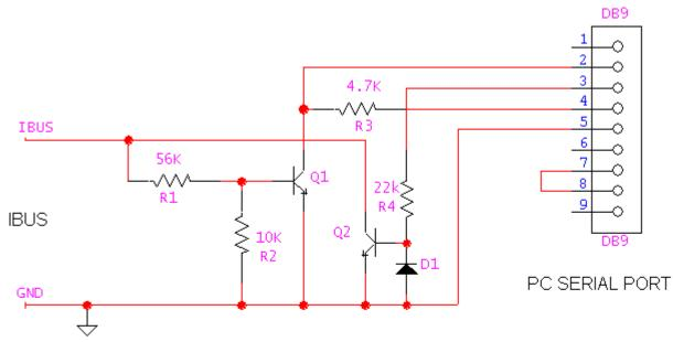
Q1,Q2 Generic NPN transistor e.g. 2N2222, 2N3904 etc
