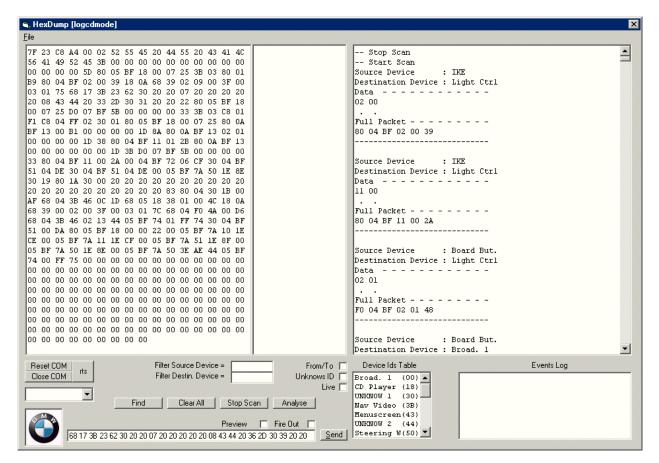
The I-Bus software analyser allows you to display I-BUS messages in clear text for everybody understanding. You have the choice to scan in real time the COM PORT and I-BUS conversations, to load a binary (.bin), an hexa file, or copy and paste to the hexa area some hexa bytes from a dump window in another software. A big part of my analysis of Ibus messages was done with that software.
